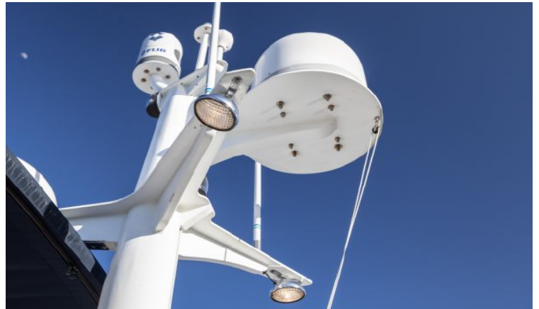
Mast with Radar and SAT TV
