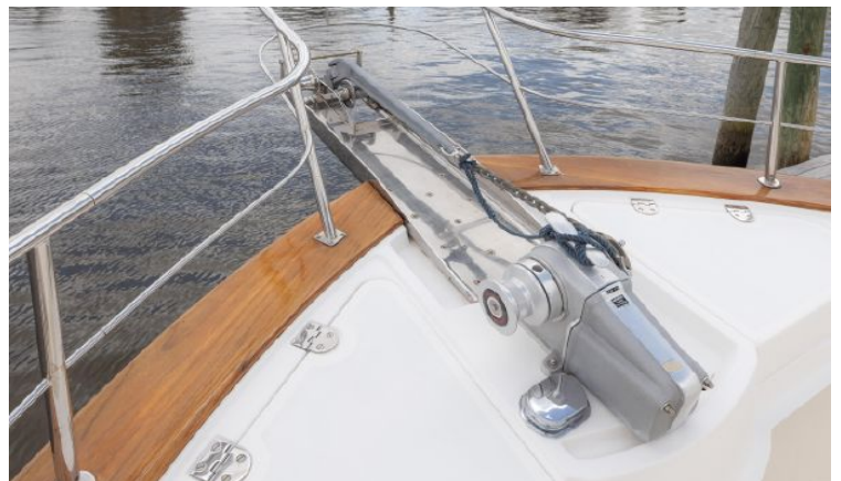
Windlass and Anchor Roller
